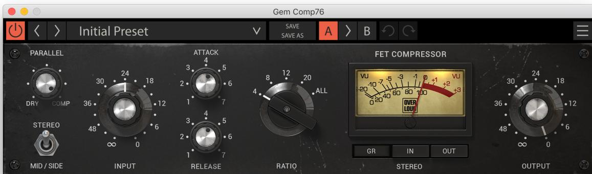
**PARALLEL** - Sets the balance between DRY and COMP (processed) sounds. This is commonly called Parallel Compression.
