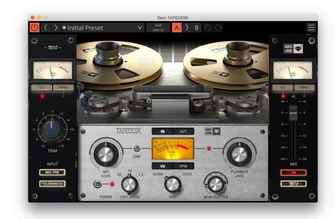
**VU METERS** - **TAPEDESK** has three Meters: two from the mixer and one in the tape machine. All three can be switched between VU or PPM modes.
