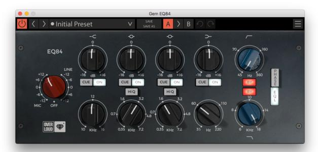
INPUT GAIN - The red knob controls the input gain using double range: MIC and LINE. Both ranges go from -12 dB to +12 dB, but the mic range also adds the modeling of the mic-preamp transformer and saturation.
