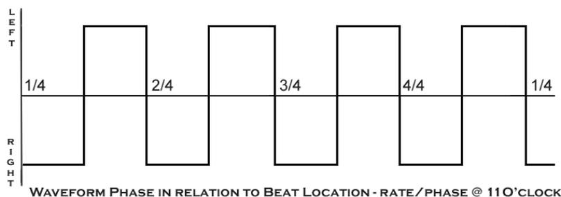
The illustration shows a square wave tremolo effect which is set to pan in stereo, synced to the host at quarter notes, so that there are four complete panning cycles per bar. In one instance, with the rate/phase knob set at 5 O'clock, the waveform is offset to the point that the signal jumps to the left channel exactly on each quarter note.
