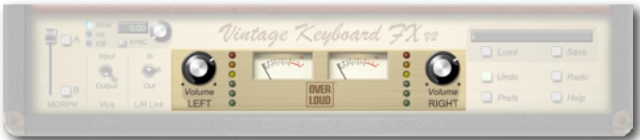
The volume knobs set the left and right channel output levels of the VKFX. The range of the volume controls is from -inf. to +15 dB.
