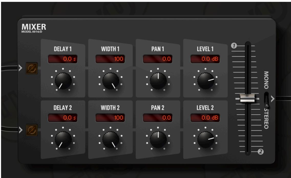
**PAN:** sets the panpot or panorama position of the input channel at the output. For stereo signal it acts as a balance control: at minimum it will only pickup the left channel signal, at maximum only the right channel will be preset at the mixer output.
